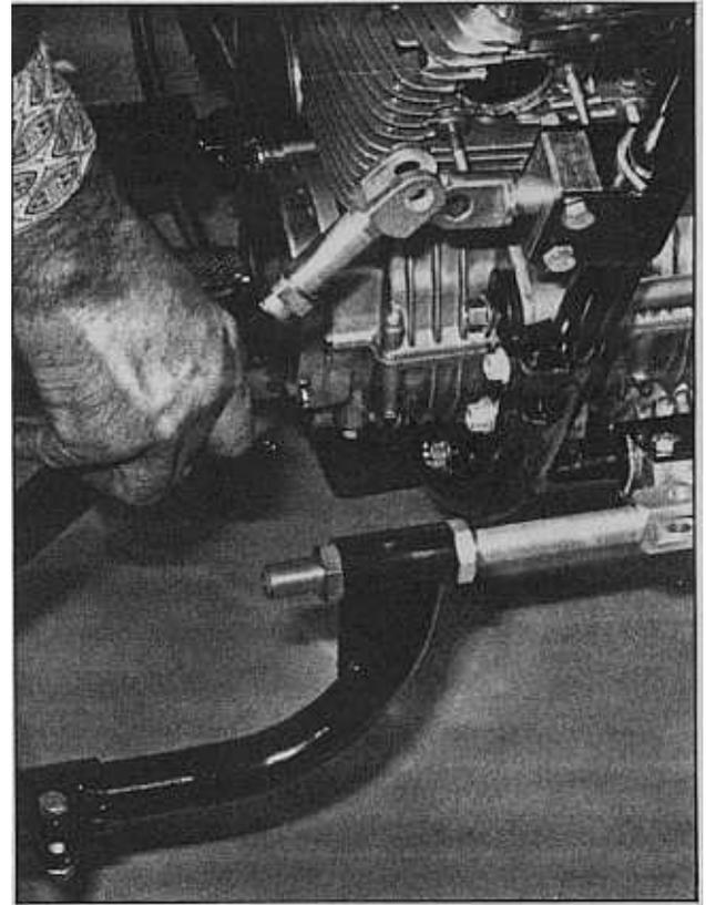
**FIGURE 4.** Clevis Adjusting Bolts must line up with Eyebolts. Note bottom front U-Clamp attached to cross tube of frame.
