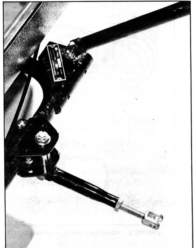
**FIGURE 5.** Rear short Strut assembled to Sliding Clamp. Eyebolts of rear long Strut assembled to sidecar frame. In all cases at least 2 inches of Clevis Adjusting Bolt must be inside Strut.
