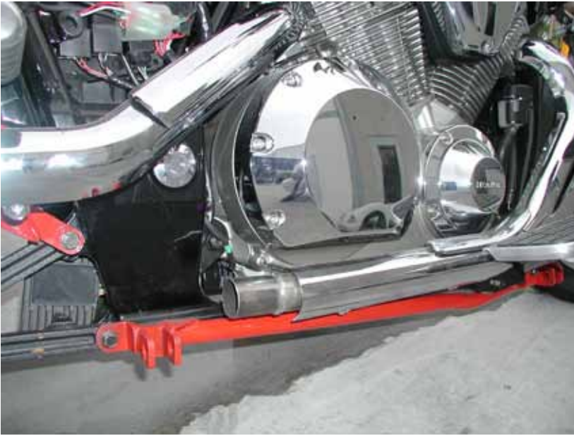
Showing bolt location to rear of sub frame
