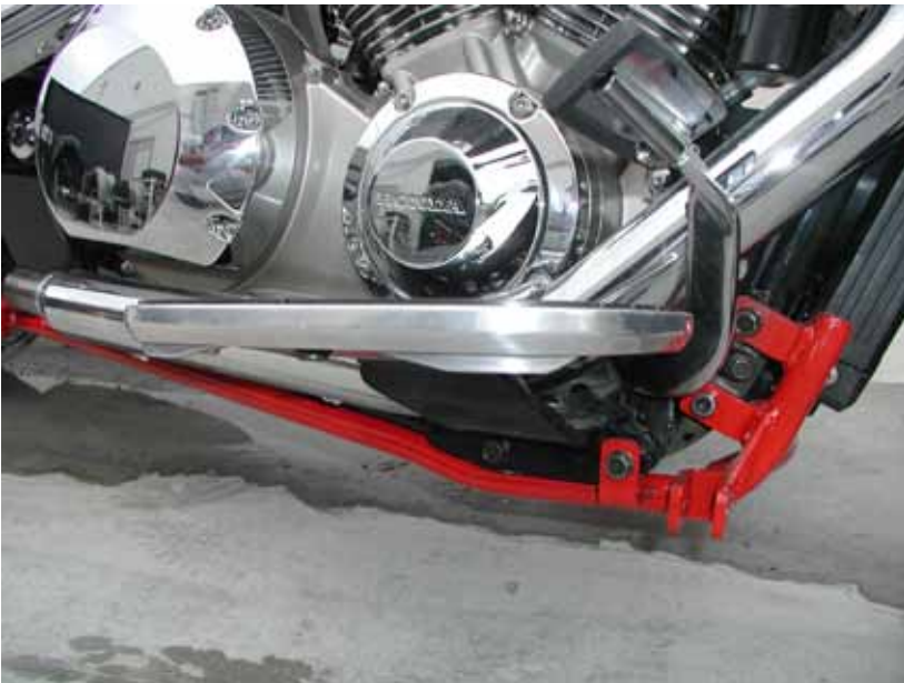
Showing bolt location to front of sub-frame
