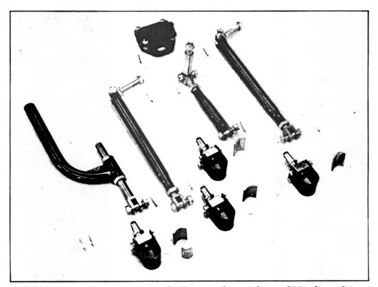
FIGURE 1. Attachment Kit, Part No. 562-08-800, showing Struts, U-Clamps, Sliding Clamp, Shims, Cotter Pins. Bolts and Nuts shown fitted to assemblies.
