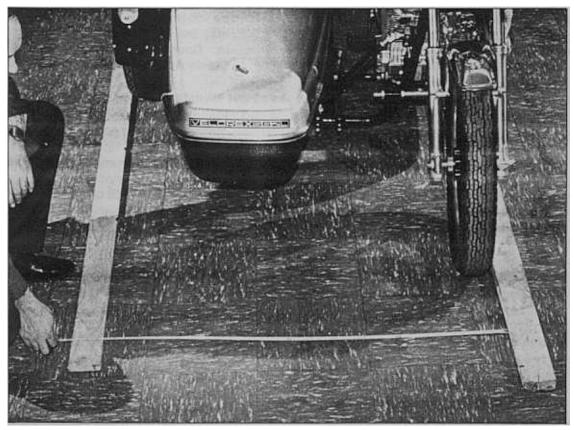
FIGURE 11. Take Toe-in measurement about one foot ahead of the front tire. Distance must be between 1/2 inch to 3/4 inches less than at rear.
