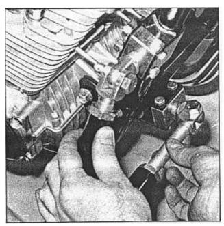
FIGURE 8. Bolts fitted to front Clevis Adjusting Bolts hold Struts in place during adjustment procedures.
