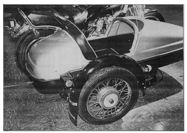
FIGURE 13. Correct wheel offset shows sidecar wheel axle 8 to 10 inches ahead of motorcycle wheel axle.
