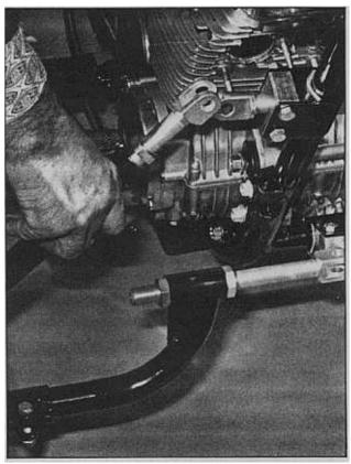
FIGURE 4. Clevis Adjusting Bolts must line up with Eyebolts. Note bottom front U-Clamp attached to cross tube of frame.
