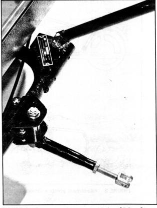
FIGURE 5. Rear short Strut assembled to Sliding Clamp. Eyebolts of rear long Strut assembled to sidecar frame. In all cases at least 2 inches of Clevis Adjusting Bolt must be inside Strut.
