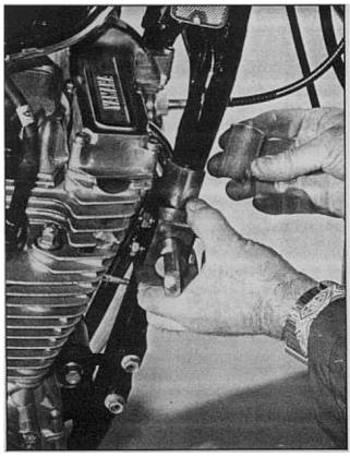
FIGURE 3. U-Clamp at top front of frame, showing large Shim in place. Small Shim in rear not needed in this case. Exhaust pipes removed for picture clarity.
