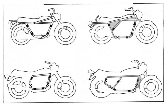
FIGURE 2. Attachment points indicated on four basic frames. X marks indicate alternate attachment points.
