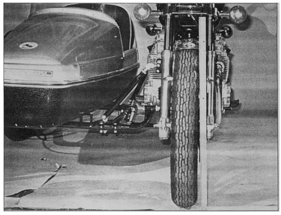
FIGURE 12. Note clearance between tire and angle bracket at ground surface. Lean-out, with empty sidecar, is 1/8 of an inch.
