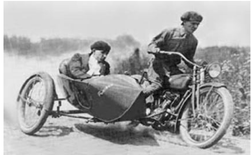
The flexible Flxible knee joint allowed the sidecar to remain level while the motorcycle rider tilted to make a turn. (Flxible Co. Photo)
